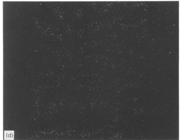
Figure 7 (a) Scanning electron micrograph of the braze joint processed at 880 °C for 30 min. (b), (c), (d) X-ray mappings of Ti, Ag and Cu, respectively, for the joint described in (a).
